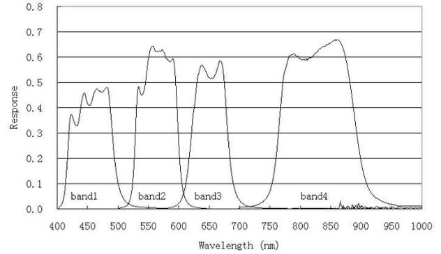
Figure 2. Actual Spectral Response of Band1-Band4
