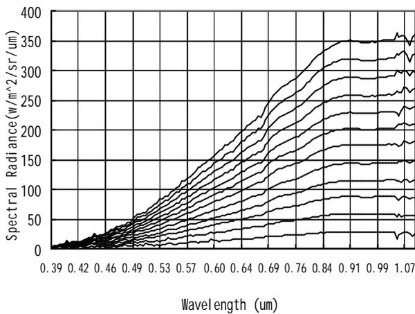
Figure 3. 12 Levels of Spectral Radiance Of Integrating Sphere
