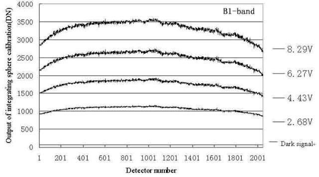
Figure.6 B1-band Output of Integrating Sphere Calibration
