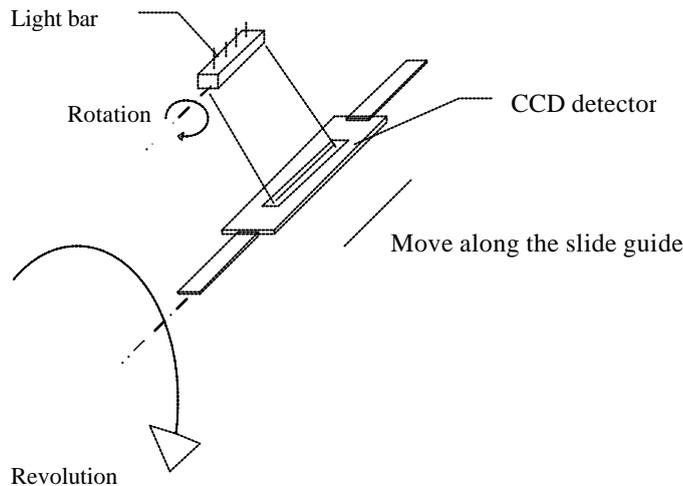
Figure 13 Experimental method of the uniformity test of irradiance in the focal plane
