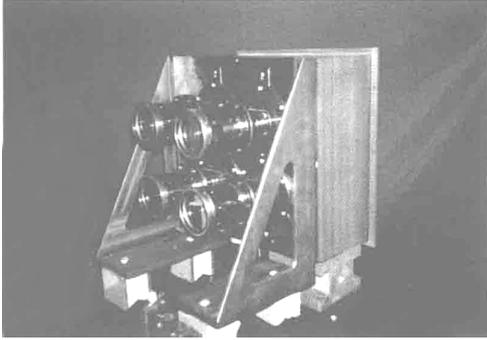
Figure 1. 4-Band CCD Camera of HY-1 Satellite
