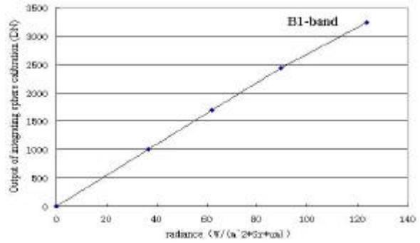
Figure.8 Linearity of Sensitivity of B1-band
