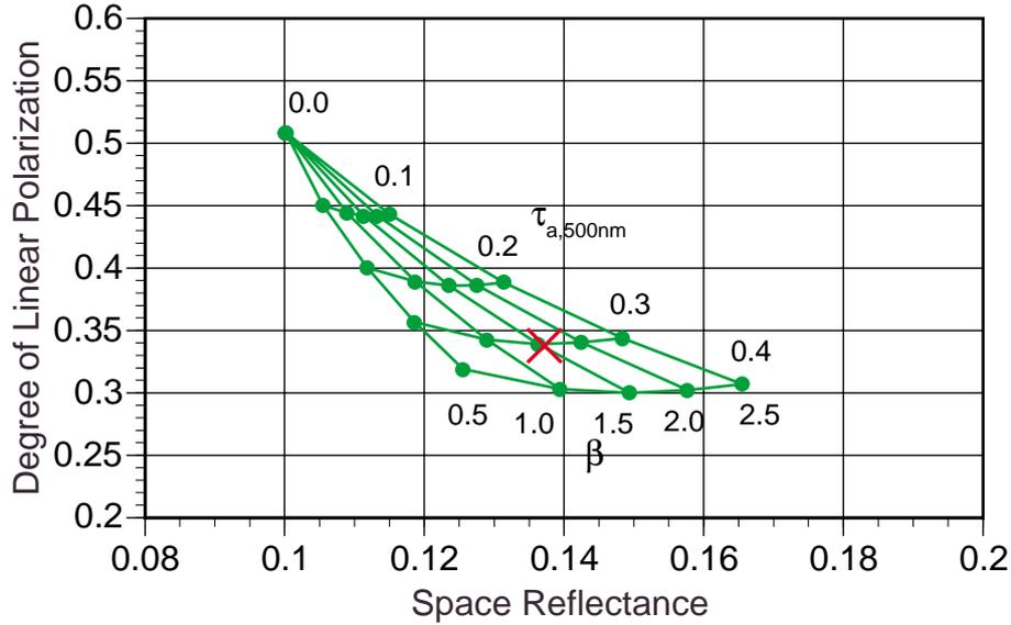
Figure2 Diagrams used by parameterized directional polarization - space reflectance in a single band; "x" represents a target area with observed reflectance and degree of linear polarization values over the desert (sand) area.
