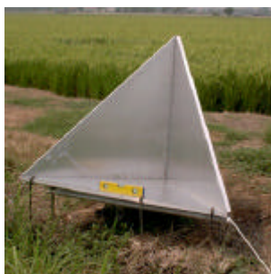
Figure 6. Field locations of corner reflectors and their corresponding views in the descending SAR image
